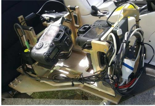
Figure 2. A photo of the acquisition rig mounted in a BushCat light sport aircraft.
